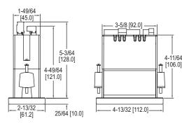
These 1/8 DIN digital panel meters accept signals from various transmitters and flowmeters and displays them on a six-digit, dual line display in engineering units. These meters will also provide power to the field device and include a NEMA 4X front panel. Free, USB based programmnig sofware is resident on the meter. Options include up to four relays and a 4-20 mA output.
