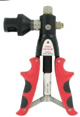
The Series PCHP Pneumatic Hand Pump comfortably sources pressure and vacuum to check calibration of gages, switches, transmitters, and recorders. The contoured cushion handles provide extra comfort while preventing the pump from sliding. The oversized check valve provides smooth operation throughout the output range. The dual o-rings on all pistons ensure zero leakage.
