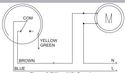
Figure 7-Filling (NC) Function FSW2-CGXX-XX
