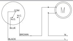
Figure 4-Double Function (Emptying (NO)) FSW2-DNXX-XX
