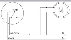
Figure 3-Filling (NC) Function FSW2-CNXX-XX
