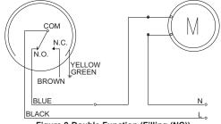
Figure 9-Double Function (Filling (NC))
