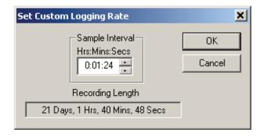
In the window above, the sampling interval was set to 1 minute, 24 seconds, to allow a 3 week recording.
