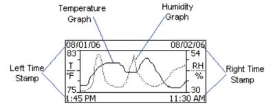
This screen shows the graph of the samples stored in logger memory. The temperature graph is shown with a solid line. The temperature axis is on the left. The humidity graph is shown with a dotted line. The humidity axis is on the right. The graph time stamps are shown on the left and on the right, above the axis.
