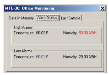
The Alarm Status pane displays the alarm thresholds for the active channels. If a high alarm occurred the threshold is displayed in red. If a low alarm occurred, the threshold is displayed in blue.
