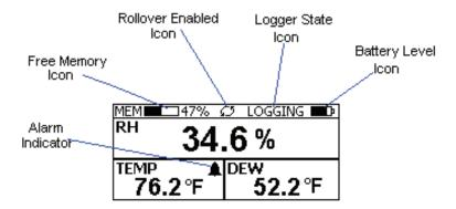
This screen shown the current Relative Humidity, Temperature and Dew Point measurements. The measurements are updated every two seconds, independent of the device sample rate.
