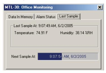
The *Last Sample* pane shows the value of the last sample taken, for all the active channels. It also shows when the next sample will be taken.
