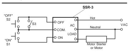
With two normally open momentary contact push buttons (S1 and S2), the SSR-3 provides solid-state control of the motor starter or the motor itself.....if load requirements are within SSR-3 ratings. S3 provides a safety shut-down. With S3 closed, the "ON" push button (S1) is rendered ineffective by the "OFF" override feature of the SSR-3
