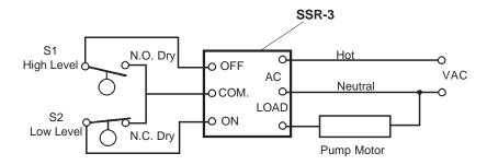
**<u>Refill</u>**: Low level permits S2 to close, starting refill pump. Rising level allows S2 to open and eventually closes S1 to actuate the SSR-3 "OFF" circuit and stop the pump motor. The SSR-3 "OFF" override assures pump shut-down even if S2 failed to open.
