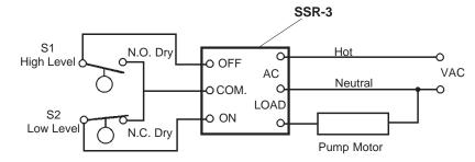
**<u>Refill</u>**: Low level permits S2 to close, starting refill pump. Rising level allows S2 to open and eventually closes S1 to actuate the SSR-3 "OFF" circuit and stop the pump motor. The SSR-3 "OFF" override assures pump shut-down even if S2 failed to open.
