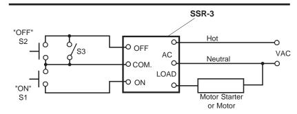
With two normally open momentary contact push buttons (S1 and S2), the SSR-3 provides solid-state control of the motor starter or the motor itself.....if load requirements are within SSR-3 ratings. S3 provides a safety shut-down. With S3 closed, the "ON" push button (S1) is rendered ineffective by the "OFF" override feature of the SSR-3
